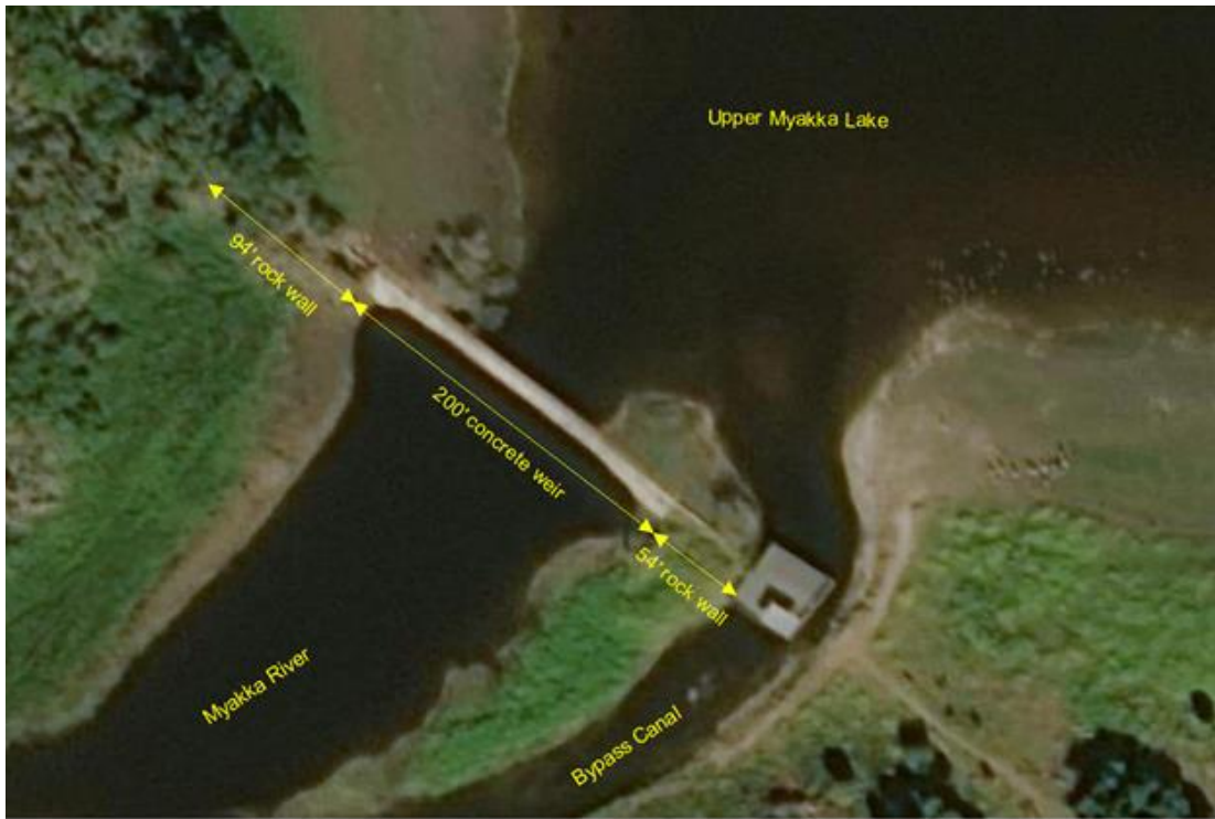
Figure 4. A 2018 aerial showing the location and measurements of the Upper Myakka Dam (8S02273) on Upper Myakka Lake in Sarasota County, FL.
